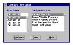
The OkiLAN 6020e will reset by selecting **OK** to save any of the options, except the *Print Configuration Sheet* option.
